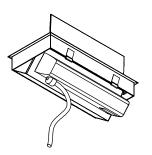
Place clips before installing in cut out.
