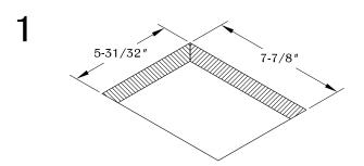
Determine the position and location of the unit on the work surface. Cut the hole at 7-7/8" X 5-31/32". Place and allow enough clearance for unit operation. DO NOT place unit where the cable is strained or trapped.
