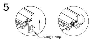
Secure unit by turning bottom wing clamp.
