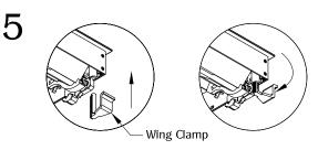
Secure unit by turning bottom wing clamp.
