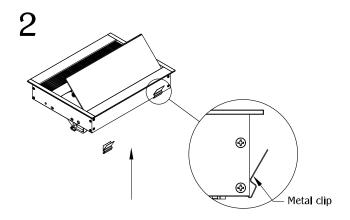
Place metal clips near the ends of the back of the unit. (NOTE: Metal clips are for use in hard surface material only as an optional mounting means.)
