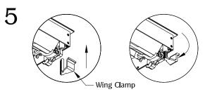
Secure unit by turning bottom wing clamp.
