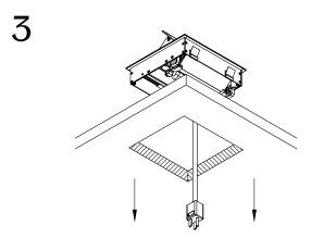
Guide the power cord through the cut out. Install the unit into the cut out and make sure it is fully leveled onto the surface.
