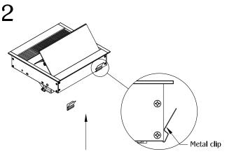
Place metal clips near the ends of the back of the unit. (NOTE: Metal clips are for use in hard surface material only as an optional mounting means.)
