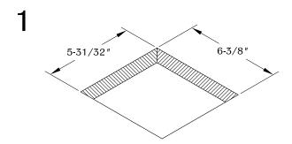
Determine the position and location of the unit on the work surface. Cut the hole at 6-3/8" X 5-31/32". Place and allow enough clearance for unit operation. DO NOT place unit where the cable is strained or trapped.
