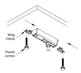
Slide the wing clamps in the underside track of the unit. Use (2) thumb screws secure the part in the work surface.
