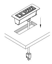
Drop the unit into the cut out. Make sure the unit is fully leveled into the work surface.
