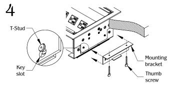
Align the mounting bracket key slots to the T-studs under the unit. Use the thumb screw to tighten and secure in place.
