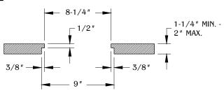
Rout out an additional 3/8" wide from under the front and rear of the cut out, providing a  $14-1/8" \times 9"$  recess. Leave 1/2" depth from the top of the cut out.
