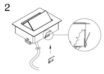
Place metal clips near the ends of the back of the unit. (NOTE: Metal clips are for use in hard surface material only as an optional mounting means.)
