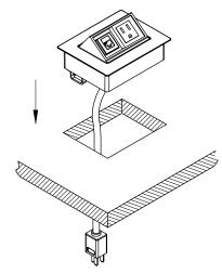
Guide the power cord through the cut out. Install the unit into the cut out and make sure it is fully leveled onto the surface.
