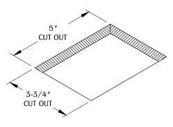
Make a cut out in the desired location on your work surface. Place near a power outlet and allow enough clearance for unit operation. DO NOT place unit where the cable is strained or trapped. Cut the hole at 5 " X 3-3/4".
