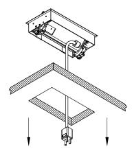
Guide the power cord through the cut out. Install the unit into the cut out and make sure it is fully leveled onto the surface.
