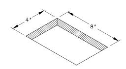
Determine the position and location of the unit on the work surface. Cut the hole at  $8" \times 4"$ . Place and allow enough clearance for unit operation. DO NOT place unit where the cable is strained or trapped.
