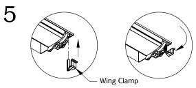
Secure unit by turning bottom wing clamp.
