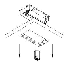
Guide the power cord through the cut out. Install the unit into the cut out and make sure it is fully leveled onto the surface.
