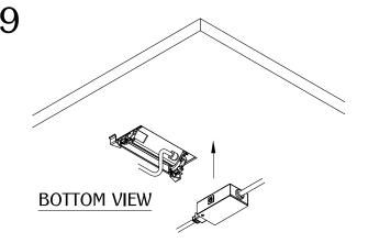
Peel the film off other side of the Hook & Loop fastener. Place the PCS/DAISYBOX on to the underside of the work surface near the unit. Make sure the indicator light is visible.
