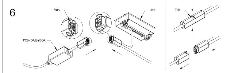
Connect the Smartlink 2.0 connectors on to the PCS/DAISYBOX and unit(s). Align the pins and snap to engage the connections. Depress the tabs on both sides and pull apart to disconnect.
