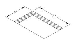
Determine the position and location of the unit on the work surface. Cut the hole at 8" X 4". Place and allow enough clearance for unit operation. DO NOT place unit where the cable is strained or trapped.
