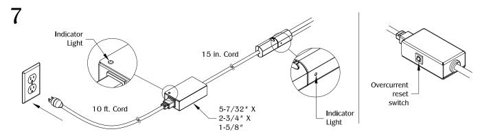
Plug in the PCS/DAISYBOX to a single 15 AMP outlet. DO NOT place where the cable is strained or trapped. The Smartlink 2.0 'indicator light' will be green or red. The Smartlink 2.0 with a "green" light means the unit is powered. It will indicate a "red" light when more than 8 units (16 MAX. power outlets total) are connected and the power will shut down. (Note: Flip the over current reset switch, when the load exceeds the rated current.)
