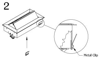
Place metal clips near the ends of the back of the unit. (NOTE: Metal clips are for use in hard surface material only as an optional mounting means.)
