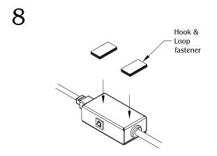
Peel the film off the Hook & Loop fastener. Apply the Hook & Loop fasteners to the PCS/DAISYBOX.
