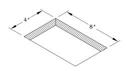
Determine the position and location of the unit on the work surface. Cut the hole at 8" X 4". Place and allow enough clearance for unit operation. DO NOT place unit where the cable is strained or trapped.
