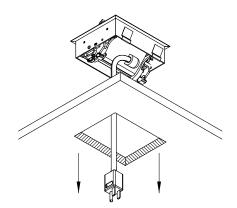
Guide the power cord through the cut out. Install the unit into the cut out and make sure it is fully leveled onto the surface.
