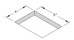
Determine the position and location of the unit on the work surface. Cut the hole at 5 " X 4". Place and allow enough clearance for unit operation. DO NOT place unit where the cable is strained or trapped.
