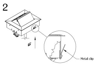
Place metal clips near the ends of the back of the unit. (NOTE: Metal clips are for use in hard surface material only as an optional mounting
