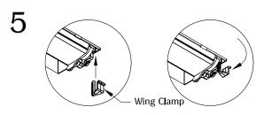
Secure unit by turning bottom wing clamp.
