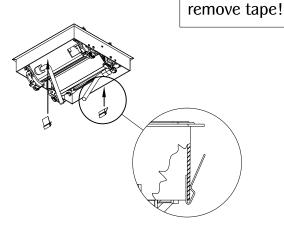
Place metal clips near the ends of the back of the unit. ( $\underline{\text{NOTE}}$ : Metal clips are for use in hard surface material only as an optional mounting means.)
