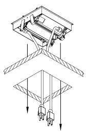
Guide the cord through the cut out. Install the unit into the cutout and make sure it is fully level on the surface.
