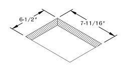
Make a cutout in the desired location on your work surface. Allow enough clearance for unit operation. DO NOT place unit where the cable is strained or trapped.
