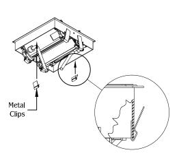
Place metal clips near the ends of the back of the unit.
