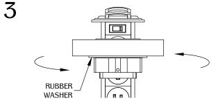
Guide the Threaded Lock ring through the power cord. Screw threaded lock ring onto mounting collar by turning clockwise. Locking ring should rotate smoothly if properly engaged. If not, the locking ring may be cross-threaded - undo and try again. Ensure rubber washer is tightly compressed against the underside of work surface.
