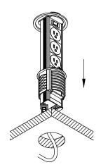
Remove the Threaded Lock Ring with the rubber washer. Guide the power cord through the cut out. Install the unit into the cut out and make sure it is fully leveled onto the surface.
