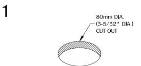
Make a cut out in the desired location on your work surface. Place near a power outlet and allow enough clearance for unit operation. <u>DO NOT</u> place unit where the cable is strained or trapped.
