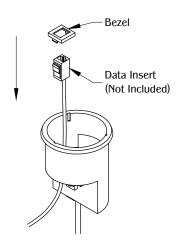
Route the data cable under the unit and through the opening. Connect the cable to the data insert. Snap the data insert to proper bezel. Snap the bezel inside the power unit.
