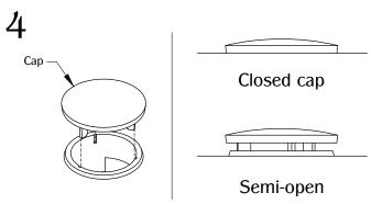
Align the cap's feet with the grooves on top of the unit to close the top. If a gap is required for wires, unalign the cap and sit the cap on top of the lip of the unit. 1
