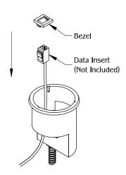
Route the data cable under the unit and through the opening. Connect the cable to the data insert. Snap the data insert to proper bezel. Snap the bezel inside the power unit.
