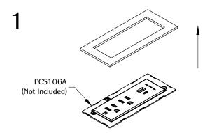
Remove the face plate on the PCS106A. (Note: PCS106A unit required.)
