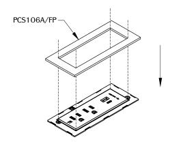
Align and snap the new face plate to the top of the unit. Make sure it is fully leveled onto the surface.
