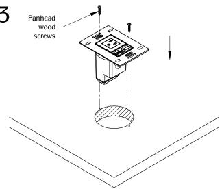
Guide the power cord through the cut out. Install the unit into the cut out and make sure it is fully leveled onto the surface. Use (2) screws to secure unit onto work surface.
