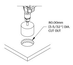
Determine the position and location of the unit on the work surface. Place and allow enough clearance for unit operation. DO NOT place unit where the cable is strained or trapped. Cut the hole at 80.00mm (3-5/32") DIA.
