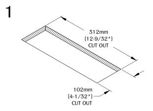
Determine the position and location of the unit on the work surface. Cut the hole at 312mm X 102mm (12-9/32" X 4-1/32").
