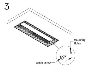
Use (2) wood screws through the mounting holes to secure on to the table top.
