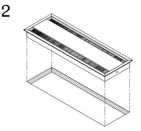
Install MAX7 into the cut out and be sure it is fully level on the surface.
