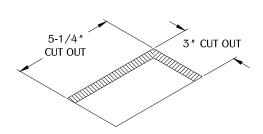
Make a cut out in the desired surface. (Note: Maximum corner radius 1/8".)
