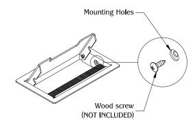
Install MAX5 into the cut out and be sure it is fully leveled onto worksurface.
