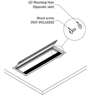
Use (2) Wood screws through the MAX12/C mounting holes to secure on to the table top.
