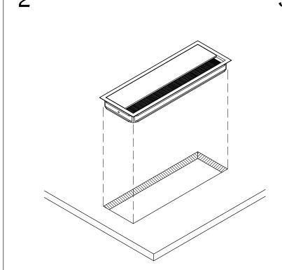
Install MAX12/C into the cut out and be sure it is fully leveled onto worksurface.
