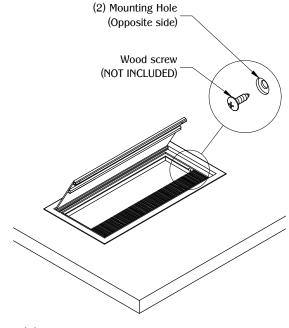
Use (2) Wood screws through the MAX12/B mounting holes to secure on to the table top.
