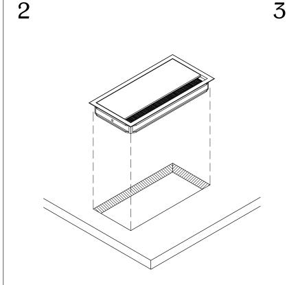
Install MAX12/B into the cut out and be sure it is fully leveled onto worksurface.
