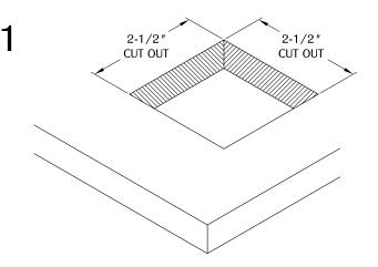
Make a cut out on the desired surface. (Note: Maximum corner radius 1/8".)
