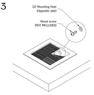
Use (2) Wood screws through the MAX11A mounting holes to secure on to the table top.
