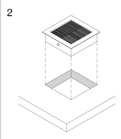
Install MAX11A into the cut out and be sure it is fully leveled onto worksurface.
