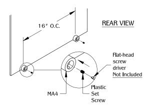
Follow the measurement in Step #2 and Install the (4) MA4 to the mirror. Secure the mirror by hand tightening the plastic set screw provided with a compatible flat-head screw driver.
