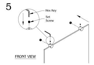
Align the mirror with the MA4 to the mounting hardware. Secure the assembly with (4) set screw.
