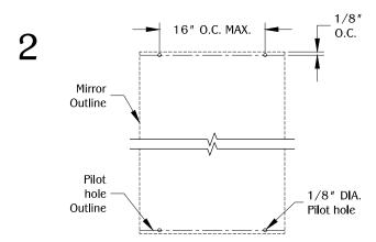
Measure 1/8" into the mirror outline and mark the desired position for the MA4. Drill (4) pilot holes recommended 16" O.C. (Note: Recommended install into studs.)
