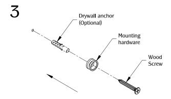
Align the (4) mounting hardware to the drilled pilot holes. (NOTE: HD-Anchor sold seperately for stronger drywall weight capacity.)
