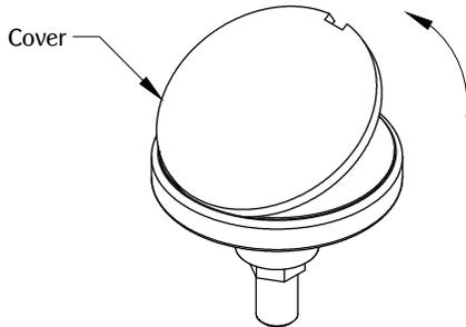
Use a flat-head screwdriver in the notch to remove cover.
