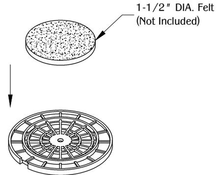
Remove cover and flip to apply felt (not included).
