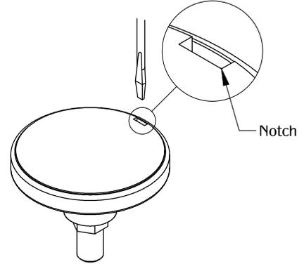
Locate the notch on the underside of the leveler.
