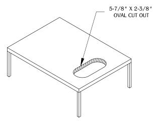
Make a cut out on the desired surface. (<u>Note</u>: We do not recommend cutting before receiving part or part sample.)
