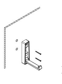
SECURE PART INTO PLACE BY INSERTING SCREWS.
