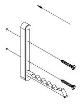
Secure the part using (2) wood screws and align the HK24 to the pilot holes.
