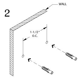
Mark and drill hole using a 9/32 "drill bit. Insert plastic anchors provided.
