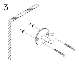
Mount backplate onto wall using the provided wood screws.
