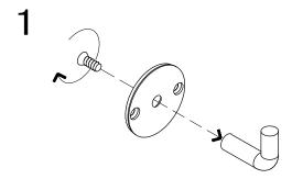
Assemble hook onto the backplate using a screwdriver.
