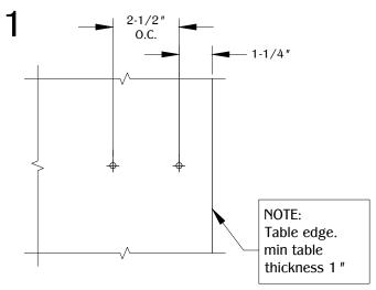
Mark screw center at 1-1/4 " from the edge of the table, mark second screw center at 2-1/2 " from center to center
