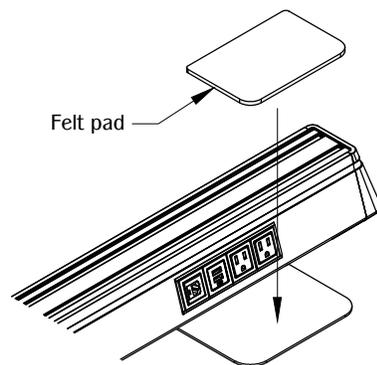
Peel the film off the adhesive backing under the felt pad. Install felt pad onto top side of landing pads.
