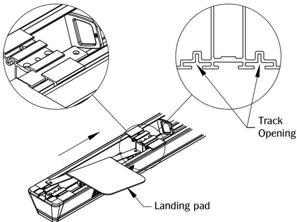
Install Landing Pad by inserting longer stem into middle track.
