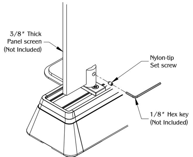
Secure panel in place by using the nylon-tipped set screw through the side of the PGRP3/F Grip as shown. (Note: Maximum panel height is 18". Recommended panel brackets should be at least 6" from the ends of each panel.)
