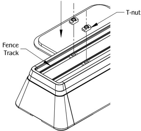
Determine desired location of PGRP3/Fence on the track. Place (2) T-nuts into the slotted track as shown.
