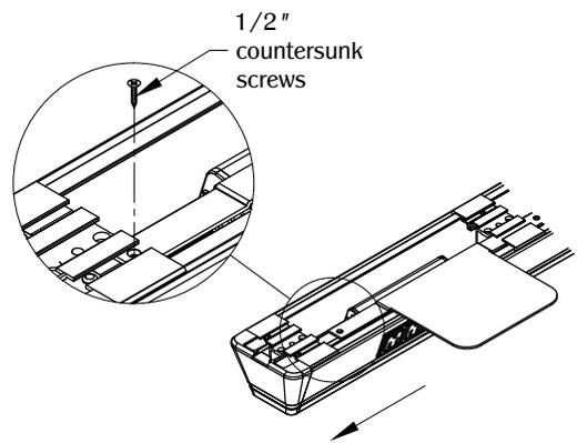
Insert shorter stem into adjacent end track and align holes on both ends. Use (2) screws to secure landing pad in place.
