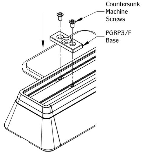
Align T-nuts with the PGRP3/F Base and secure in place using (2) countersunk machine screws.
