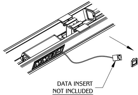
Feed cabling through the open data port and install your data insert into the designated bezel from data tree (see Note on Page 1). Route the cable through the underside of the unit.
