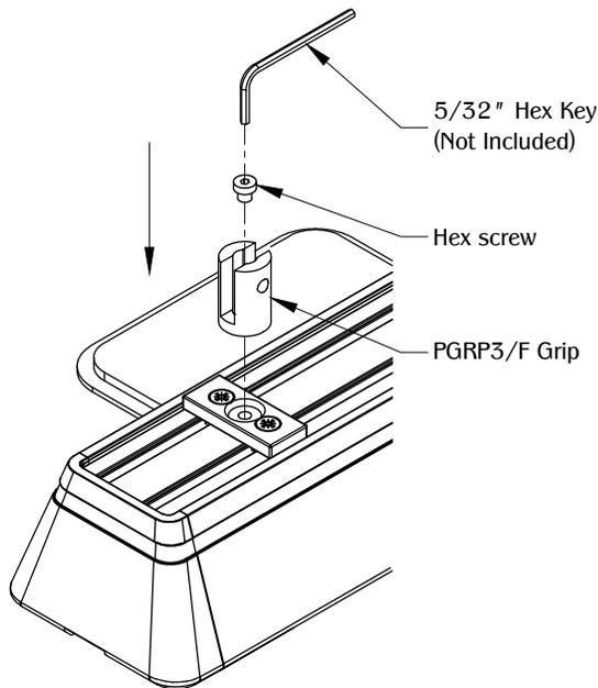
Install PGRP3/GRIP into the center countersunk cavity on the PGRP3/F Base. Secure in place with the hex screw. (Note: Repeat Steps 1-3 for all other panel bracket sets as needed.)
