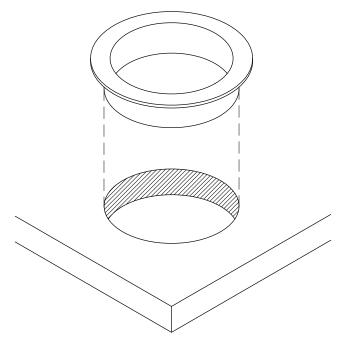
Install EDP1 into the cut out and be sure it is fully leveled onto worksurface.
