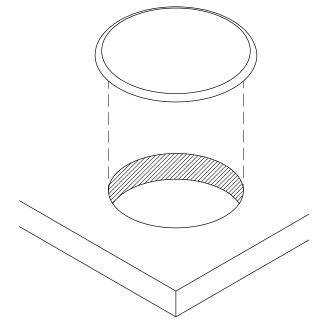
Install EDPW2 into the cut out and be sure it is fully leveled onto worksurface.
