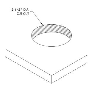
Make a cut out on the desired surface. (<u>Note:</u> We do not recommend cutting before receiving part or part sample.)
