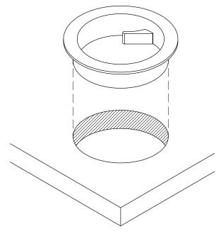
Install EDPCG1 into the cut out and be sure it is fully leveled onto worksurface.
