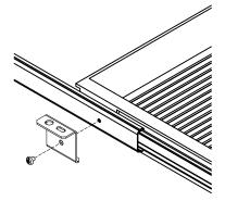
Connect (4) Mounting Brackets to slide track with (4) machine screws.
