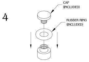
Attach the rubber ring to the mounting base and secure it by using the cap.
