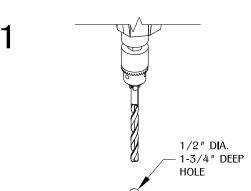
Drill 1/2" DIA. hole at 1-3/4" deep for concrete installation (Note: proceed to Step 3 for wood floor installation).
