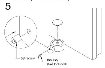
Install the cap on top of mounting base. Secure cap by using a hex key to tighten set screw.
