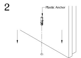
Install the plastic anchor into pre-drilled hole.
