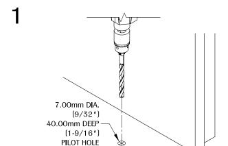
Determine the position and location of the part in the work surface behind the door. Mark the mounting position and drill the pilot hole.
