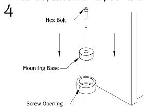
Align base and rubber stop to plastic anchor. Make sure set screw opening is lined up on both pieces. Secure the assembly with the hex bolt.
