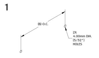
Determine the position and location of the part in the work surface. Mark the mounting positions and drill the pilot holes for the mounting hardware.
