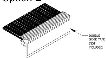
Mount BREXT onto desired surface using double-sided tape (not included).
