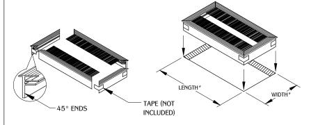
Cut brush and extrusion to desired lengths and hold together using tape. Make cut out onto desired surface and insert.
