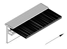
Insert brush strip into extrusion.
