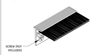
Mount BREXT onto desired surface using screws (not included).
