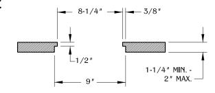
From the bottom of the table route out the A sides by an additional 3/8" wide, providing a  $14-1/8" \times 9"$  hole. Leave 1/2" depth from the top on both sides.
