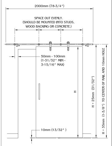
Lay out your bar accordingly and drill the holes for the rail. Rail brackets must be installed into studs, wood backing or concrete. Do not install rail brackets into dry wall only!
