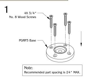
Place PGRP3 Base onto desired work surface. Make sure it is fully leveled onto the surface. Secure using (4) 3/4" No. 8 wood screws.
