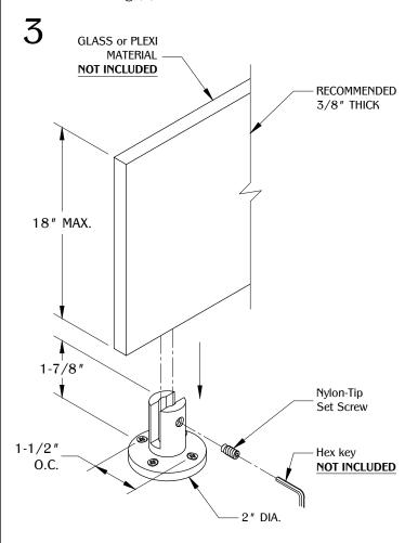
Align the 3/8 " material to the PGRP3 Grip. Secure the material with the (1) 5/16 " nylon-tip set screw.
