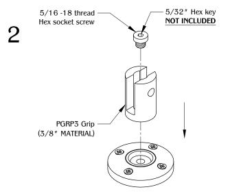
Place PGRP3 Grip on top of PGRP3 Base and fasten with the (1) 1/4" 5/16 - 18 thread hex socket screw.
