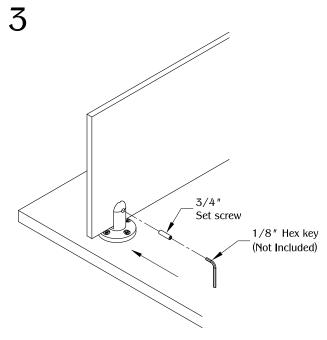
Secure the panel by using a 1/8" hex key to tighten the 3/4" set screw. (Note: Nylon-tip set screw available for glass panel installation. Sold separately.)
