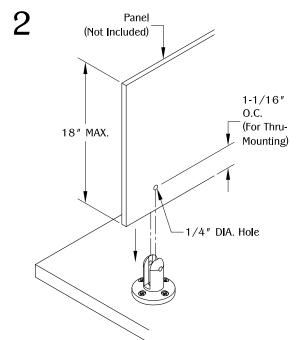
Drill a 1/4" diameter hole at 1-1/16" on center from the bottom of the panel material. Install and align pre-drilled panel hole to the panel bracket.
