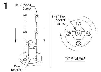
Determine the position and location of the part on the work surface. Make sure the PGRP1B is fully leveled onto the surface. Secure by using (4) No. 8 wood screws. (Note: Use a hex key to adjust panel bracket to desired orientation.)
