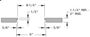
Rout out an additional 3/8" wide from under the front and rear of the cut out, providing a 14-1/8" x 9" recess. Leave 1/2" depth from the top of the cut out.
