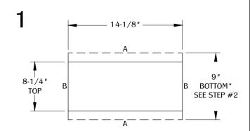
Determine the position and location of the unit on the work surface. Cut the hole at 14-1/8 " X 8-1/4 " from the top.
