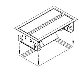
Install the unit into the cut out and be sure it is fully level on the surface.
