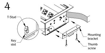
Align the mounting bracket key slots to the T-studs under the unit. Use the thumb screw to tighten and secure in place.
