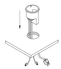
Install the unit into the cut out and make sure it is fully level on the surface. (Note: For a tighter fit in to the cut out, apply tape around the outside perimeter of the unit.)
