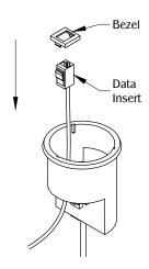
Route the data cable under the unit and through the opening. Connect the cable to the data insert. Snap the data insert to proper bezel. Snap the bezel inside the power unit.
