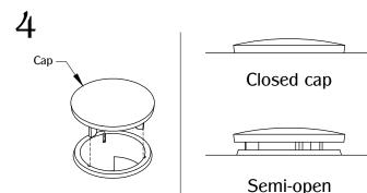
Align the cap's feet with the grooves on top of the unit to close the top. If a gap is required for wires, unalign the cap and sit the cap on top of the lip of the unit. 1
