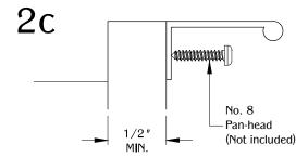
Center the part on the top front drawer panel and secure with (2) mounting screws.
