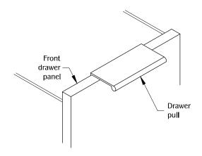
Determine the position and location of the part in the work surface. Center the part on top of the front drawer panel.
