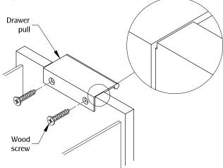
Install the part flushed into the routed surface. Secure with (2) mounting screws.
