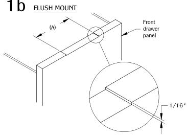
Determine the position and location of the part in the work surface. Rout the top of the front drawer panel. (See page 1 chart for length.)
