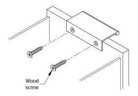
Secure with (2) mounting screws. (Note: Mounting holes and hardware varies by size see chart.)
