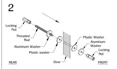
Assemble the base with (1) locking nut, (1) threaded rod, (1) aluminum washer and (1) plastic washer at the back of the work surface. Align the assembly through the predrilled hole. Repeat the same assembly order from the front side.
