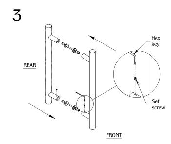
Align the DH5 to the assembled base. Secure it with the (4) set screw using the hex key.
