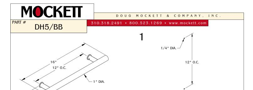
Determine the position and location of the DH5 at the work surface. Drill a 1/4" diameter hole with the recommended on center dimension.
