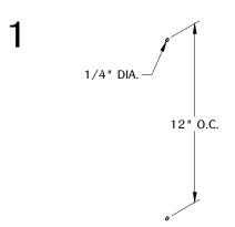
Determine the position and location of the DH4 at the work surface. Drill a 1/4 " diameter hole with the recommended on center dimension.
