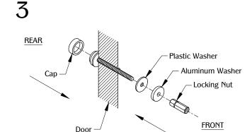
Assemble (1) aluminum washer, (1) plastic and (1) locking nut washer at the front of the work surface. Tighten the assembly. Finish the hardware assembly by installing the cap. Repeat Step 3 & 4 for the other side.
