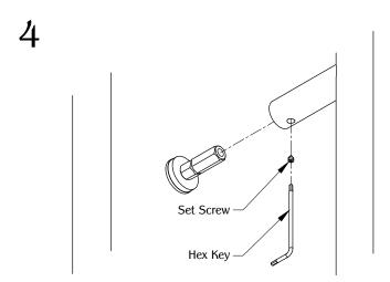
Align the DH4 to the assembled base. Secure it with the (2) set screw using the hex key.
