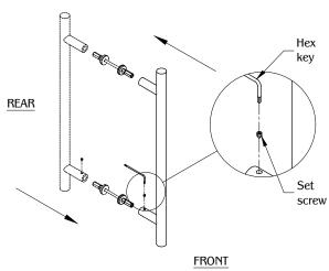
Align the DH4 to the assembled base. Secure it with the (4) set screw using the hex key.
