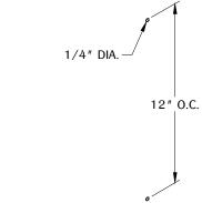
Determine the position and location of the DH4 at the work surface. Drill a 1/4" diameter hole with the recommended on center dimension.
